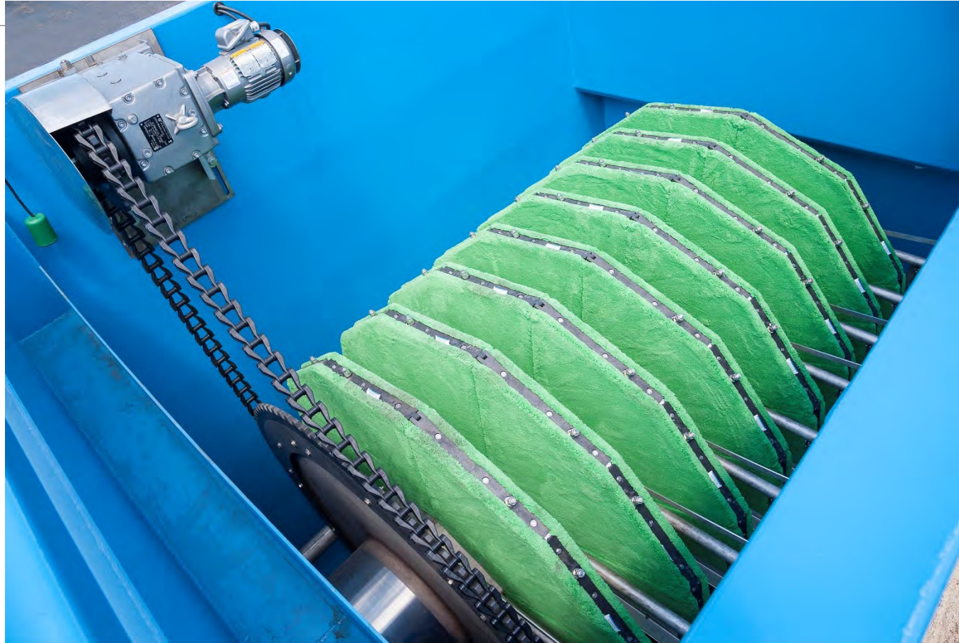
First full-scale (3 MGD) AquaPrime® Filter demonstration
